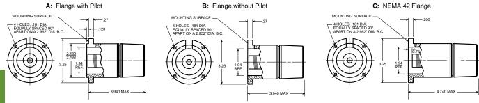
**Mating shaft lengths:** Typically: 0.5" max. available into the coupling as measured from the A/B mounting surface. 1.3" max. available into the coupling as measured from the C mounting surface.
