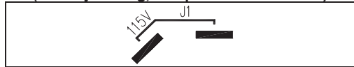
Figure 2 - Control Set for 230 Volt AC Line Input (Factory Setting, Jumper J1 Not Installed)
