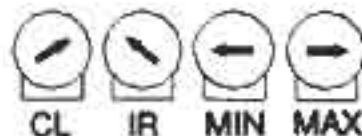
FIG. 1 - FACTORY SETTING OF TRIMPOTS
