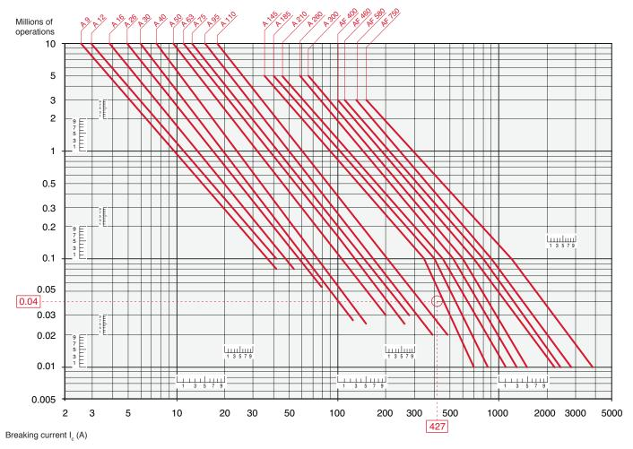
Motor power 59 kW for AC-4 -  $U_e$  = 600 V utilization – Electrical durability required = 0.04 million operations. As stated on page 0/0: 59 kW, 600 V corresponds to  $I_e = 71.1$  A.
