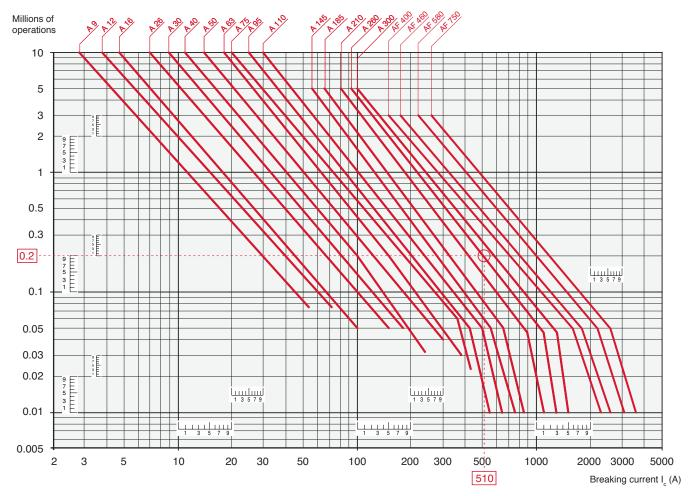
Motor power 45 kW for AC-4 - U<sub>a</sub> = 400 V utilization – Electrical durability required = 0.2 million operations. 45 kW, 400 V corresponds to I<sub>g</sub> = 85 A.
