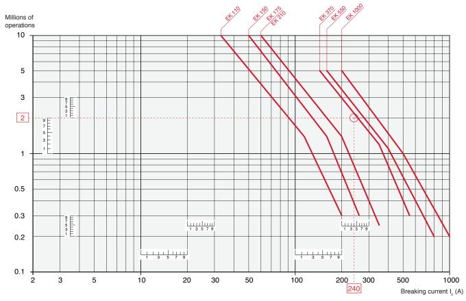
Example:  $I_c / AC-1 = 240 A - Electrical durability required = 2 million operations.$  Using the AC-1 curves above select the EK 370 contactor at intersection "O" (240 A / 2 million operations).
