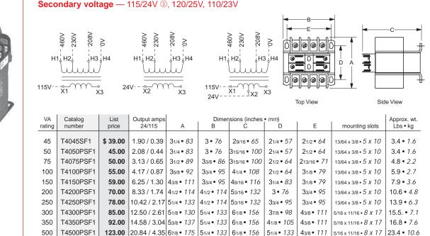
NOTE: Primary & secondary fuse block provided as standard (except for the 45VA unit where only the secondary fuse clip is provided.
