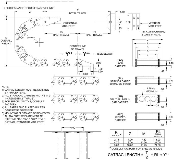
\*\* IF THE STATIONARY FOOT IS MOUNTED ON EITHER SIDE OF THE CENTER LINE OF TRAVEL, THE DISTANCE (Y) BETWEEN CENTER LINE AND STATIONARY FOOT MUST BE ADDED TO CATRAC LENGTH.
