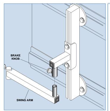
UNIVERSAL MOUNTING SYSTEM Attachments slide easily onto swing arm or base posts. No tools required. Knob locks attachment in place following adjustment. Kits-Include Base, Arms & Attachment
