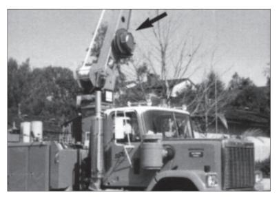
**GLEASON K-REEL** installed on a hoist.
