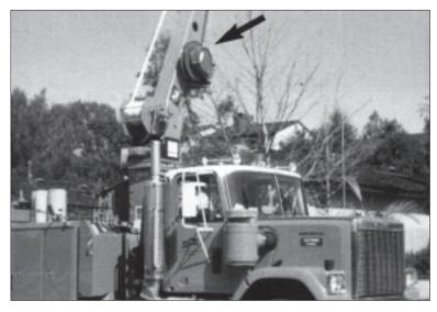
GLEASON K-REEL installed on a hoist.
