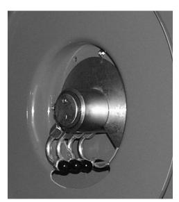
"Goose-necks" plus integral ramp assure smooth hose transition between manifold and reel spool.
