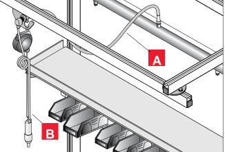
The most flexible air line we have found. Ideal for connecting tool trolley to manifold or other supply because its flexibility does not interfere with trolley movement. Clear, reinforced plastic, 3/8" I.D. with 3/8" NPT male swivel fittings on both ends.
