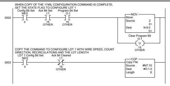
When the LDT configuration data has been acknowledged for LDT 1, the program will copy the configuration data for LDT 2 into the output image table. The speed of wire is defined as  $9.272\mu$ s/inch. The counts will be increasing from the LDT head. There is one recirculation in the LDT and the LDT length is 24.0 inches. This will continue until the command is acknowledged by the 1746L LDT Interface Module.
