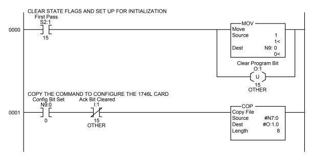
When the configuration command is complete, the program will copy the LDT configuration command for LDT 1 into the output image table with the programming bit set. This command will configure LDT 1 for the speed of wire, count direction, recirculations, and LDT length. The speed of wire for LDT 1 is  $9.300\mu$ s/inch. The counts are defined as increasing from the LDT head. There is only 1 recirculation and the LDT length is 12.0 inches. This continues until the command has been acknowledged.
