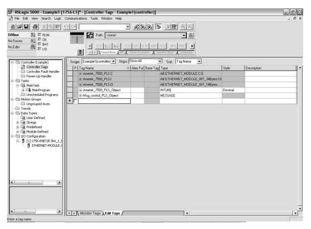
After the message tag is created, edit the tag properties of the MESSAGE tag and click on the configure button next to the data type:
