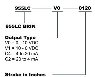
Insert stroke in inches to 0.1 inch. Enter as a fourplace number. **Example:** 12.0 in stroke entered as 0120. To convert a metric stroke to inches, multiply millimeter value by 0.03937.
