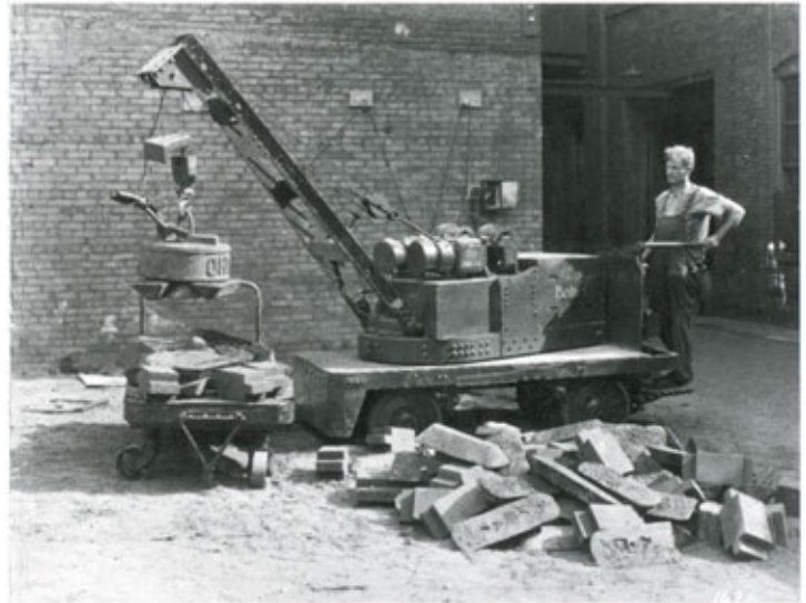
Lifting pig iron ingots with 20" Ohio Magnetics magnet Baker Tractor & Truck Co. - 1917
