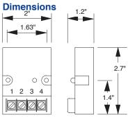
**Connections** The MCS operates with the Load in series with the timer. A Load must always be connected in series with the MCS to avoid damage.
