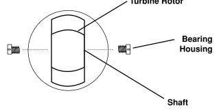
\* Note that on ceramic shaft models the shafts are in the screws and the bearings are in the rotor. Follow the same basic procedure above. (#25945)
