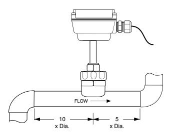
Horizontal is the preferred installation orientation, since it improves low-flow performance and avoids problems with trapped air. Bottom, top, and vertical pipe installations are all acceptable if required by the piping layout.
