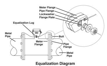
Run wire from equalization lug to both pipe flanges; secure flange plates under bolt heads as shown.
