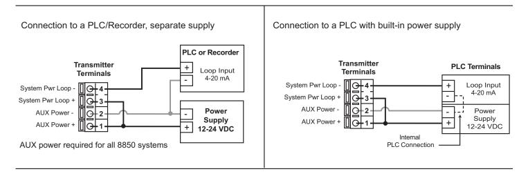
Example: Two transmitters connected to PLC/Recorder with separate power supply
