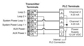
Example: Two transmitters connected to PLC/Recorder with separate power supply
