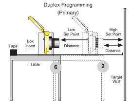
Position the switch at the desired HIGH HIGH set point distance defined as the air gap space between the transducer and the target. Make sure that the switch is stationary and perpendicular to the target before continuing.
