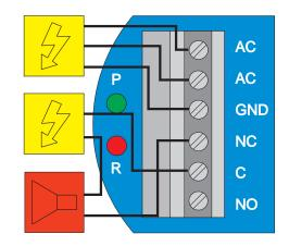
**Warning:** The use of an appropriate motor starter or secondary relay is recommended with pumps, valves or alarms to prevent damage to the relay contacts. The use of suppressors (snubbers) is strictly recommended when switching inductive loads.
