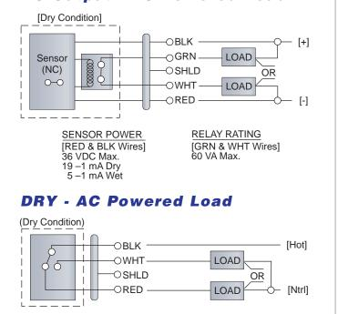
SENSOR WIRING NO - WHT & BLK Wires NC - RED & BLK Wires SENSOR RATING -13\_1: 120 VAC/VDC @ 15 VA
