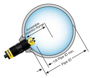
When using any type of fitting, the orientation as well as the insertion depth of the flow switch in the pipe is critical. See the diagram below for the recommended orientation depth.
