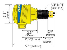
**Set Points:** The AT1\_-\_63\_ series liquid flow switch set point is factory calibrated to 0.2 fps and the AG1\_-\_36\_ series gas flow switch is set to 10 fps. To convert feet/sec to GPM, please refer to the chart below.
