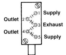
The 4 way 5 port air valve offers direct sequential operation of air cylinders, air motors, etc., or for air logic circuits. The valve is supplied with barbed fittings for 1/4" O.D. flexible tubing and is directly interchangeable with the spacing of one electrical switch.
