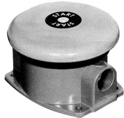
The Type D Mushroom Button foot and palm operated switches contain 1 or 2 contact blocks, as selected, and these are mounted with terminals or manifold up for good accessibility. The operating button, which is the switch cover, is securely fastened to the enclosure by the indicating plate located in the center of the operating button. Removal of the nameplate and operating button provides access to the contact block assemblies.
