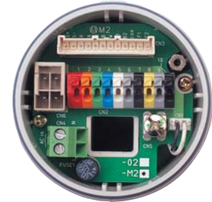
Color Coded Wiring Terminals
