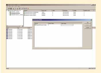
You can easily check and control your PLCs with QUICK CLIENT software. It allows you to test your PLC connection, toggle I/O, read/write values and test ASCII strings in real time while sitting comfortably at your PC.
