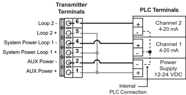
Example: Two transmitters connected to PLC/Recorder with separate power supply
