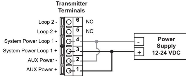
Connection to a PLC/Recorder, separate supply
