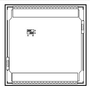
In this figure, the jumper settings will cause the inputs to function as npn, 24VDC digital inputs
