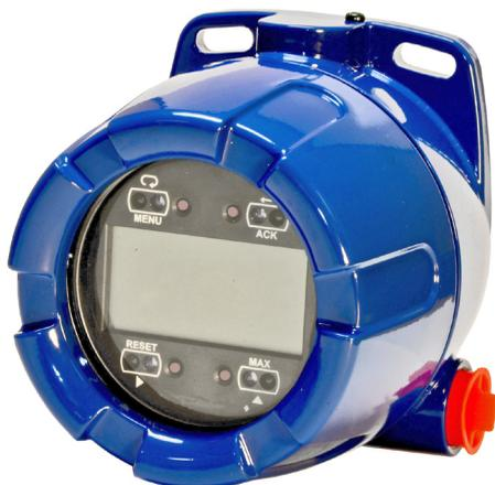
CSA approved explosion proof loop powered level indicator brings modern design, easy readability and enhanced functionality to hazardous environments displaying engineering units connected in series with one 4-20 mA, continuous level transmitter. Select this level indicator for hazardous applications with an explosion proof level sensor. The windowed field enclosure is wall mounted.
