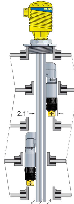
A key feature of Smart Trak™ is the adjustability of the level switches. When two level switches are placed close together, one of the switches will need to be moved to allow for the switches to be staggered into the installation fitting. Once installed, the level switch can be returned to its required position.
