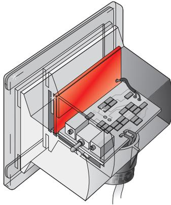
The general purpose non-intrusive capacitance level switch provides reliable liquid level detection of water based conductive liquids with non-coating and/or scaling characteristics with a 1A relay output. Media examples include hydrochloric, sulfuric acid and water. The liquid level sensor is bracket mounted on the exterior wall of non-metallic tanks and applied as a high level alarm or low level alarm.
