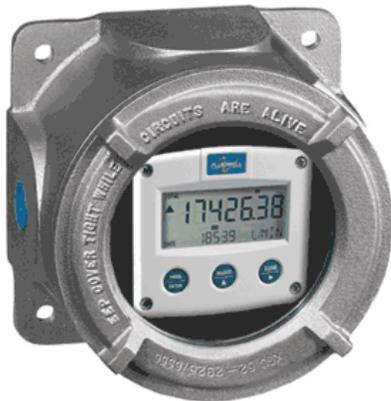
CSA approved explosion proof for hazardous environments, the loop powered level indicator displays engineering units connected in series with one 4-20 mA continuous level transmitter. Select this level indicator for hazardous applications with an explosion proof level sensor. The windowed field enclosure is wall mounted.
