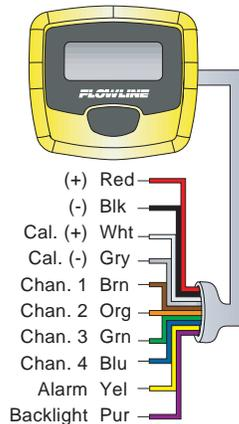
**C. Sensor Cable:** The maximum cable distance between the indicator and attached Flowline transmitter, level or leak detection switch is 1000 feet (304m). Use a well insulated and shielded twisted pair cable sized from 14-18 gauge.
