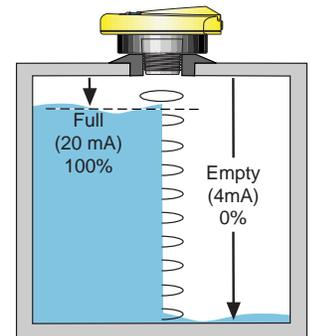
**C. MicroCal Calibration:** To customize engineering units, configure FET alarm set points from level transmitter, level switch or leak detection switch inputs, and/or linearize the volumetric measurement of odd shaped tanks, use the MicroCal calibration kit. **MicroCal calibration users should now go to the MicroCal Calibration Kit LI96 Series Owners Manual for programming instructions. Once calibrated, return to this manual and continue starting with the Installation Section.**
