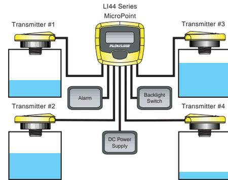
**A. Factory Calibration:** Out of the box, the indicator is factory calibrated to interface with (4) SOURCING two-wire loop powered level transmitter inputs and display percentage of measured span on each channel. The following describes the indicator functions as delivered under factory calibration:
