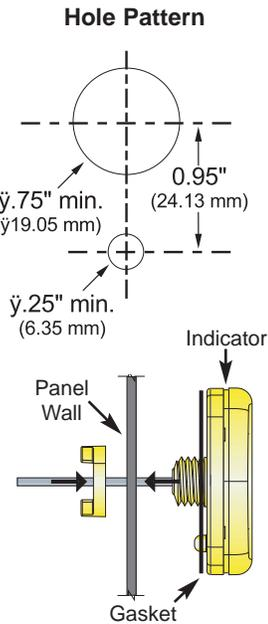
**C. Wall Mount:** Follow the below steps to install the indicator in a wall mount configuration:
