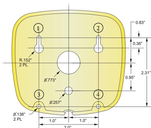
Use the above hole dimensions for purposes of drilling the (4) wall bracket mounting holes.
