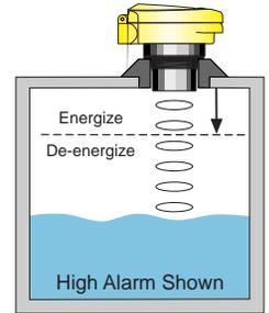
**High and Low Level Out of Bounds Alarm:** Programmed with two set points, the high and low level out of bounds alarm protects the top of the tank from overspill and the bottom of the tank from run-dry. If the level rises above or falls below the set points, the relay will energize. The relay will remain de-energized as long as the level is in between the set points.
