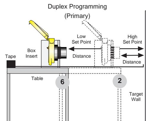
11. Position the switch at the desired HIGH HIGH set point distance defined as the air gap space between the transducer and the target. **Make sure that the switch is stationary and perpendicular to the target before continuing.**
