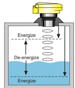
**Automatic Fill or Empty:** Programmed with two set points, the latched automatic fill or empty will control a pump or valve. When the level reaches the energize set point, the latching relay will energize, and remain energized until the level reaches the de-energize set point.
