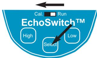
**E. Selecting a Relay Channel:** After entering the CAL mode, press the SELECT button once and the Relay 1 LED will turn ON indicating that the channel is now active for set point calibration. Press the SELECT button again until the desired Relay channel becomes active.
