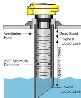
4. **Stand Pipe:** A stand pipe may be used to dampen turbulence or separate surface foam. Select a 2" or larger pipe for models LU75-5\_ \_5 and LU72-5\_ \_5. Select a 3" or larger pipe for models LU71-5\_ \_5 and LU73-5\_ \_5. The pipe length should run the measurement span. Cut a 45° notch at the bottom of the pipe and drill a 1/4" pressure equalization hole high in the dead band.
