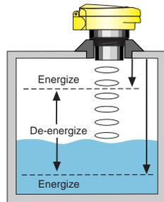
2. Position the switch at the desired HIGH set point distance defined as the lesser of the two air gap spaces between the transducer and the target. **Make sure that the switch is stationary and perpendicular to the target before continuing.**
