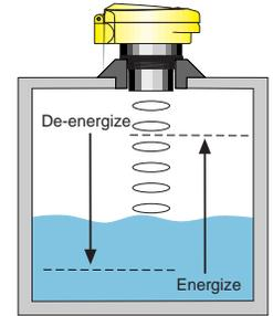
2. Position the switch at the desired LOW set point distance defined as the greater of the two air gap spaces between the transducer and the target. **Make sure that the switch is stationary and perpendicular to the target before continuing.**
