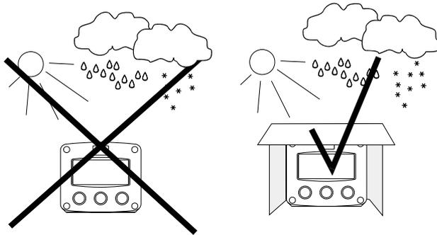
Take the relevant IP classification of the casing into account (see manufactures plate). Even an IP67 (NEMA 4X) casing should NEVER be exposed to strongly varying (weather) conditions.
