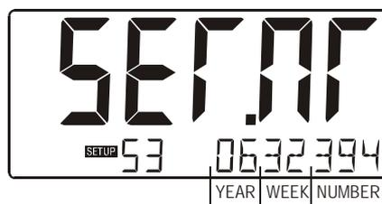
Fig. 7: Example serial number.
