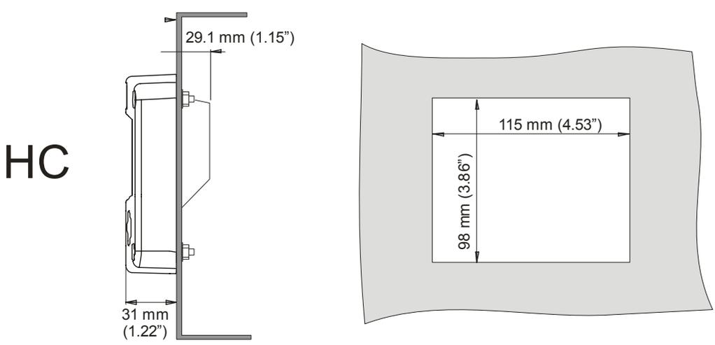
Fig. 5: Dimensions GRP enclosures.
