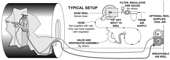
**E**□**ZPULL CLEAN AIR REELS** include stainless steel air path. Also includes ball stop and ratchet lock. Finish is OSHA safety blue baked-on polyester. 3/4"-16 UNF fitting to fit MSA #455022 hose or equivalent. **Does not include hose.**
