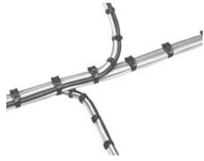
Sample cable tie installations
