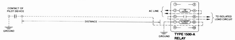
Single conductor remote control using ground return.
