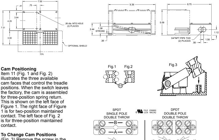
(Fig. 3) Remove the screw in the center of the cam block. Lift the cam block straight up. Allow the cam follower to rise with the block. When the cam block is up as high as it will go, tip it as shown in Fig. 3 and remove. Turn the cam block to provide the desired face as described on Cam Positioning paragraph above. Install the cam block observing the procedure described above.
