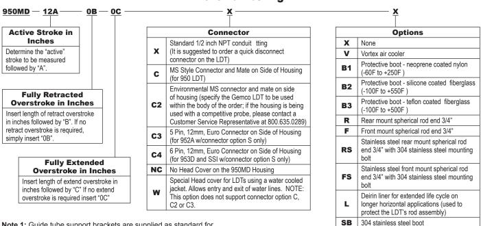
**Note 1:** Guide tube support brackets are supplied as standard for strokes of 72" or greater.
