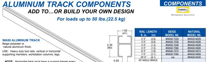
NOTE: Horizontal track must have a support hanger every 6.0 ft.(1.8m) to maintain maximum rated capacity.
