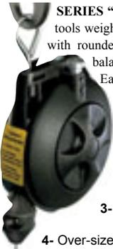
**SERIES "BD" TOOL BALANCERS** are the economical choice for balancing tools weighing up to 5 lbs(2.3kg). Molded ABS housing has a smooth exterior with rounded edges designed for maximum ergonomic appeal. Series "BD" balancers are the most modern, easiest to adjust, and reliable available.
