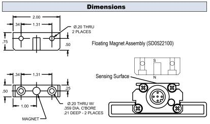
NOTE: The north pole of the magnet should be pointed towards the probe.
