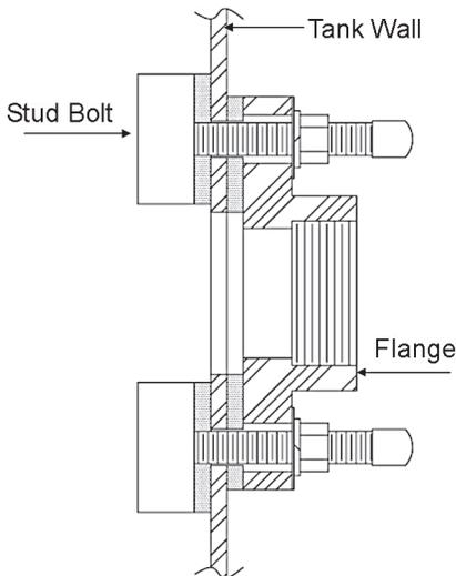
Bolted Flange Bulkhead Fitting
