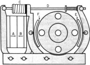
When the twin magnets (A and B) become de-energized, spring C simultaneously moves tie rod D to the left and magnet B to the right, forcing both brake shoes (E and F) to apply brake torque to the wheel at the same time.
