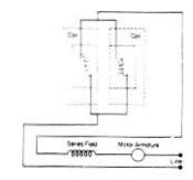
**Figure 4: Series Coil Connection**
